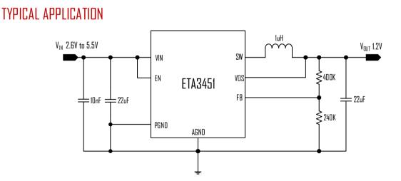
Typical Application Circuit of 1.2V Output
