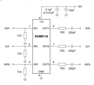
Figure 1. Input DC Coupling and Output AC Coupling Application Schematic
