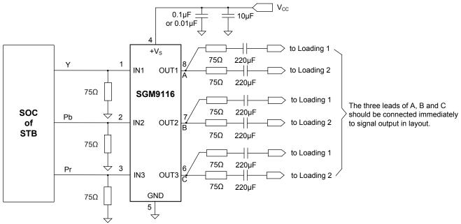
Figure 2. Input DC Coupling and Output AC Coupling Application Schematic in STB
