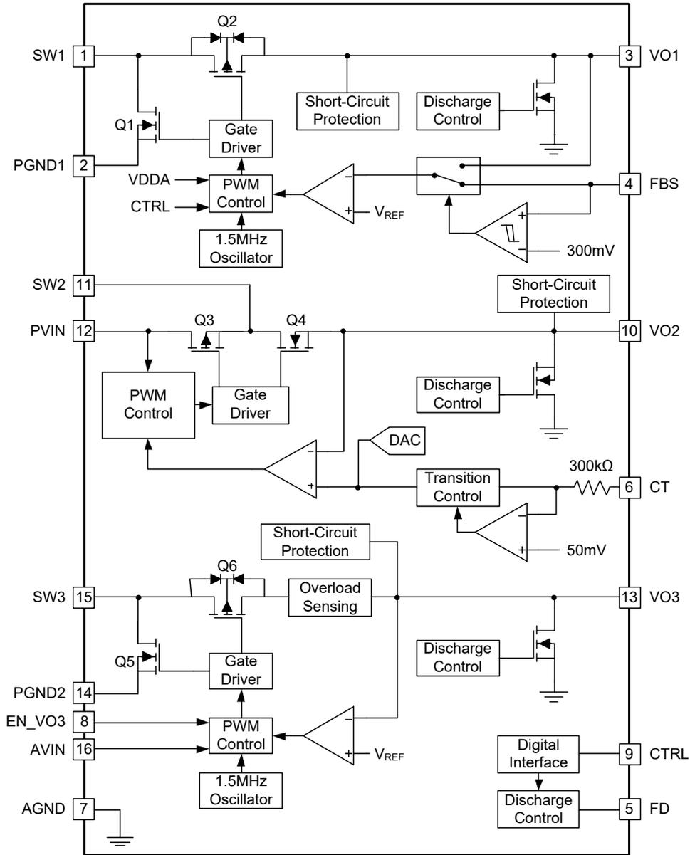
Figure 3. SGM3836A Functional Block Diagram
