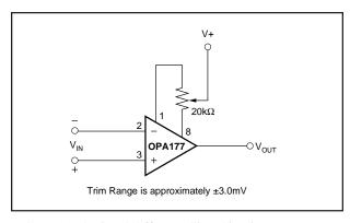
FIGURE 1. Optional Offset Nulling Circuit.
