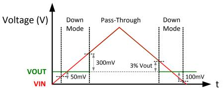
Figure 12. Down Mode and Pass-Through Operation
