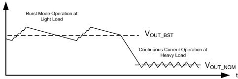
Figure 11. Burst Mode Operation
