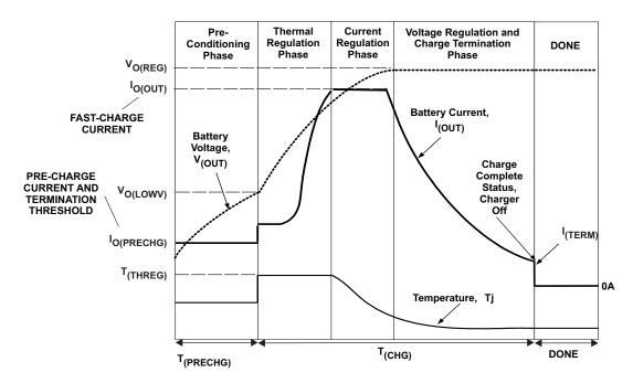
图 8. Charging Profile With Thermal Regulation
