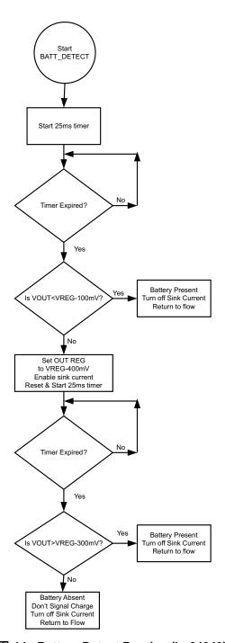
图 14. Battery Detect Routine (bq24040)
