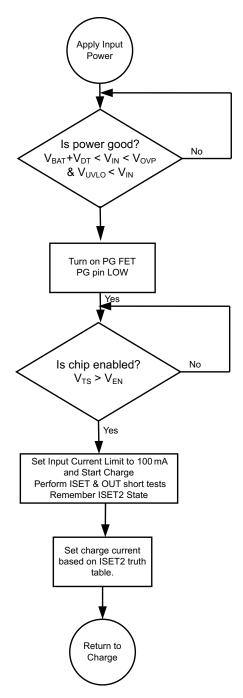
图 10. bq2404x Power-Up Flow Diagram
