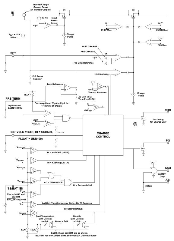
图 7. Functional Block Diagram
