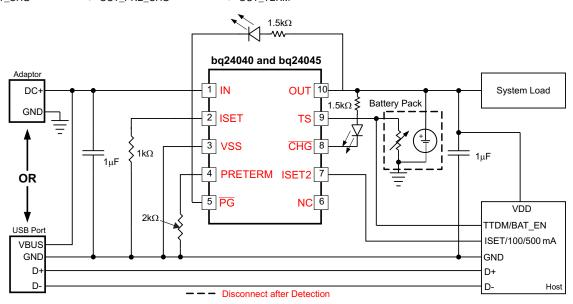
图 15. Typical Application Circuit: bg24040 and bg24045
