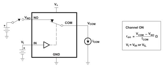
Figure 11. ON-State Resistance (r<sub>on</sub>)
