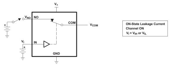
Figure 13. ON-State Leakage Current ( $I_{COM(ON)}$ ,  $I_{NC(ON)}$ )
