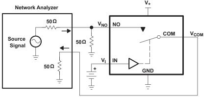
Channel OFF: NO to COM  $V_I = V_+ \text{ or GND}$
