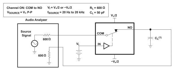
(1) C<sub>L</sub> includes probe and jig capacitance.
