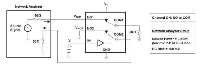
Figure 17. OFF Isolation (O<sub>ISO</sub>)
