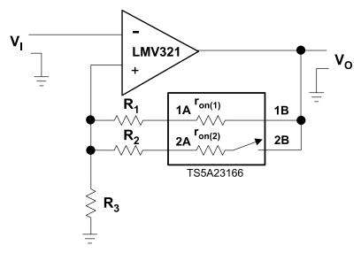
Figure 21. Gain-Control Circuit for OP Amplifier
