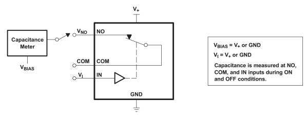
Figure 14. Capacitance (C<sub>I</sub>,  $C_{COM(OFF)}$ ,  $C_{COM(ON)}$ ,  $C_{NC(OFF)}$ ,  $C_{NC(ON)}$ )
