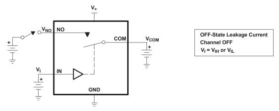
Figure 12. OFF-State Leakage Current ( $I_{COM(OFF)}$ ,  $I_{NC(OFF)}$ ,  $I_{COM(PWROFF)}$ ,  $I_{NC(PWR(FF))}$ )
