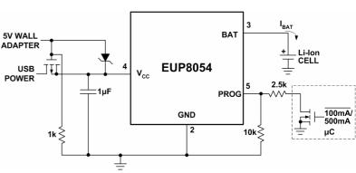
Figure 1. 600mA Single Cell Li-ion Charger
