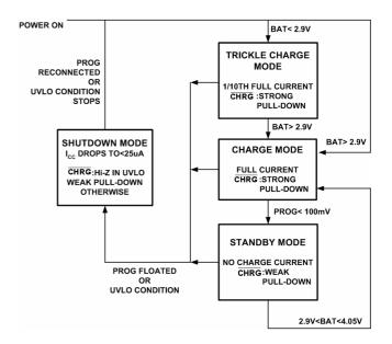
Figure 7. State Diagram of a Typical Charge Cycle
