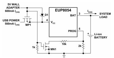
Figure 12. Combining Wall Adapter and USB Power
