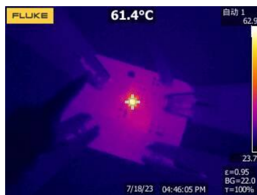
Figure 20. Thermal, VIN=5V, VOUT=1.2V, ILOAD=3A
