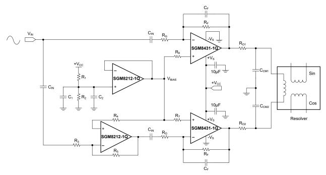
Figure 2. Resolver Excitation Circuit with SGM8212-1Q
