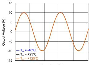
Time (40µs/div) Figure 6. Output Voltage of Resolver Excitation Circuit
