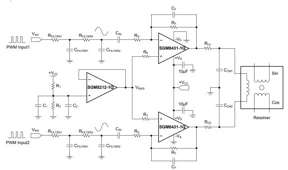
Figure 4. Resolver Excitation Circuit from PWM Input Signal
