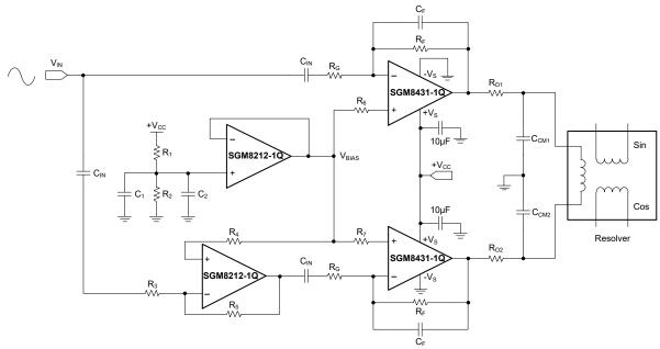
Figure 1. Resolver Excitation Circuit
