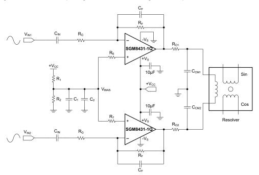
Figure 3. Simplified Resolver Excitation Circuit without SGM8212-1Q
