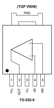
NOTE: The PAD should be connected to  $\ensuremath{\text{-V}}\xspace_{S}$  , and the wiring must be as short as possible.
