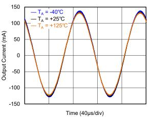
Figure 7. Output Current of Resolver Excitation Circuit
