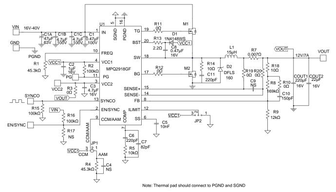
Figure 14: 12V Output Typical Application Circuit for TSSOP Package (Vout = 12V)
