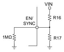
Figure 4: EN/SYNC Resistor Divider
