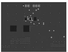
Bottom Layer Figure 11: Recommended PCB Layout for QFN Package (7)
