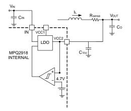
Figure 7: Configuration of VCC2 Connecting to  $V_{\text{OUT}}$
