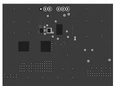
Bottom Layer Figure 10: Recommended PCB Layout for TSSOP Package <sup>(6)</sup>
