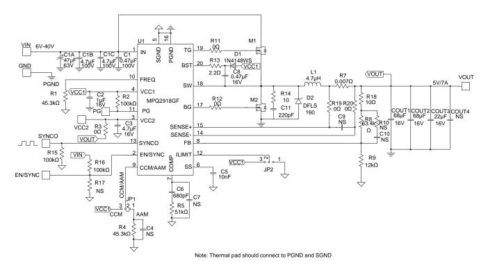
Figure 13: Typical Application Circuit for TSSOP Package (VOUT = 5V)
