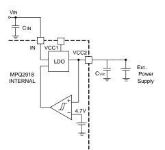
Figure 6: Internal Circuitry of VCC2
