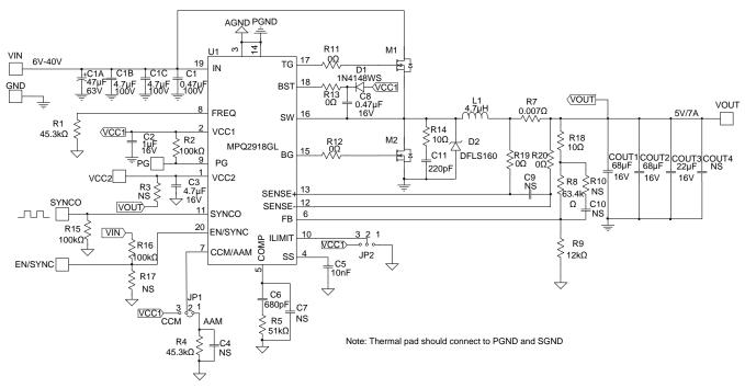
Figure 15: 5V Output Application Circuit for QFN Package
